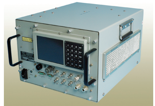
Mark XIIA IFF interrogator for naval, land-based air defense, airborne surveillance, and air traffic control applications
