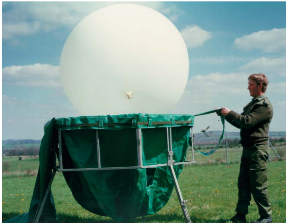
BMETS includes ground meteorological instrumentation and balloon inflation and launching device (BILD)
