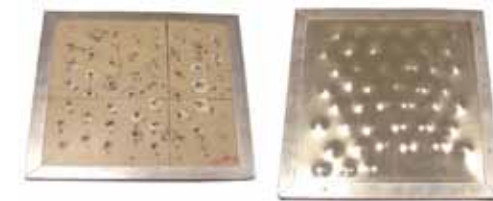
Test panel shot 45 times – no complete penetrations (front and rear views)
