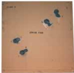
Level 3 target after two sets of four 7.62 mm APM2 impacts to STANAG 4569 spacing
