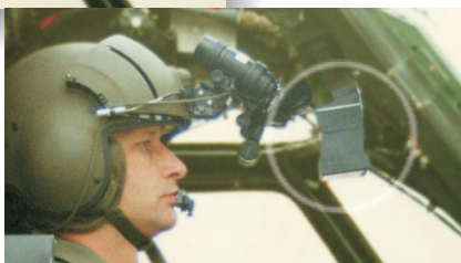
MonoHUD installation with night vision goggles in place or raised
